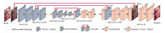
Figure 3: Self2Self architecture figure from [23]. It implements a simple U-Net structure and takes a  $B \odot y$  and predicted the masked region  $(1 - B) \odot y$ .
